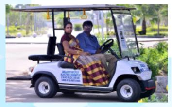
Dr. R. Seyezhai, from the department of Electrical and Electronics Engineering (EEE), and her PhD student, Mr. A. Bharathi Sankar have designed a 4 seat battery powered vehicle which can be charged by solar radiation and electricity. The big innovation in the creation of this vehicle has been the development of advanced electric drive using brushless DC motor, an industry first. The vehicle can cover up to 70 kilometres at a maximum speed of 40 km/hr on a single charge.
